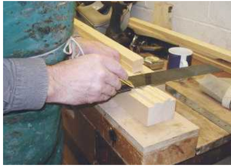
▲ Pic.11 After planing and moulding the stiles and rails, the stiles are marked...
